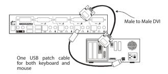
Repeat steps 1a and 1b or and 2 to connect the remaining computers to the available ports. Devices and computers that are connected to SV431DVIUA can now be turned on.
